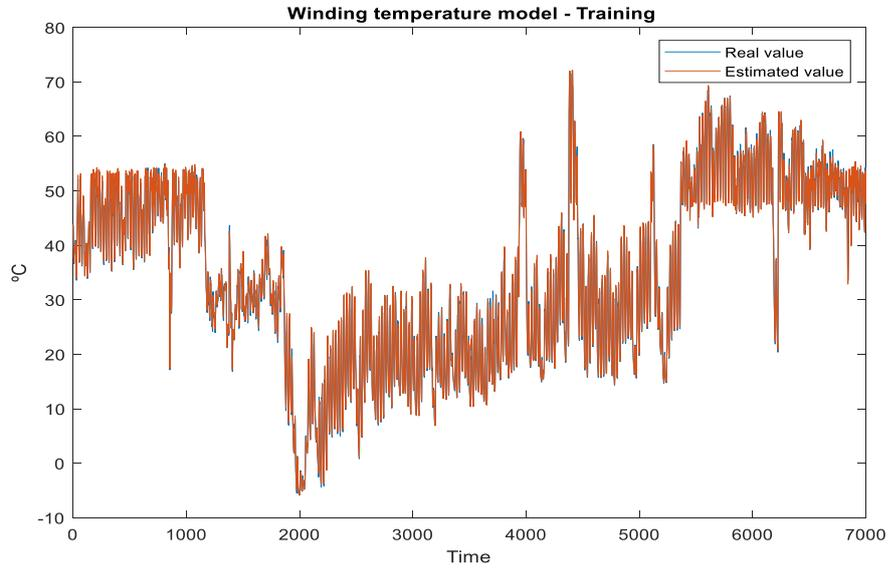
FIGURE 12 RESULTS OF THE WINDING TEMPERATURE MODEL FOR PT-2
