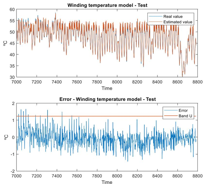
FIGURE 13 EVALUATION OF THE WINDING TEMPERATURE MODEL FOR PT-2
