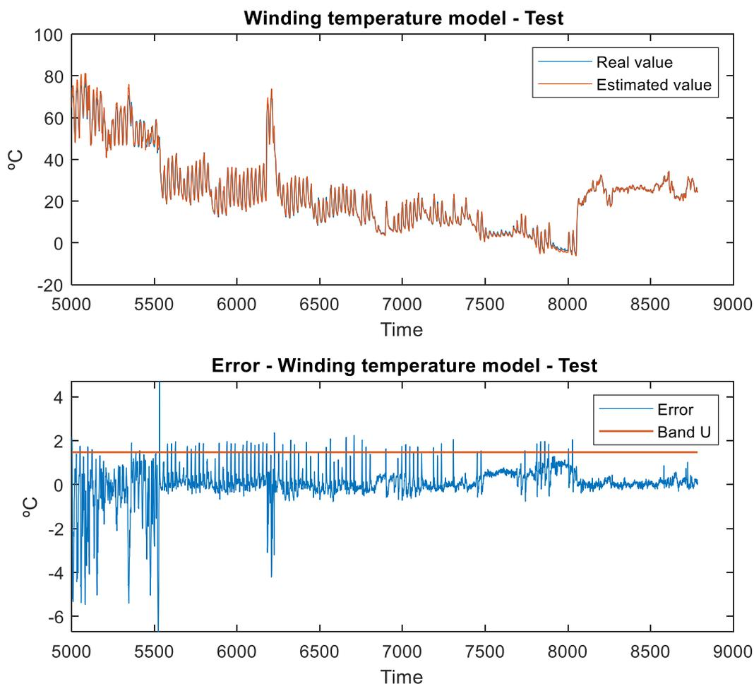
FIGURE 15 EVALUATION OF THE WINDING TEMPERATURE MODEL FOR PT-1
