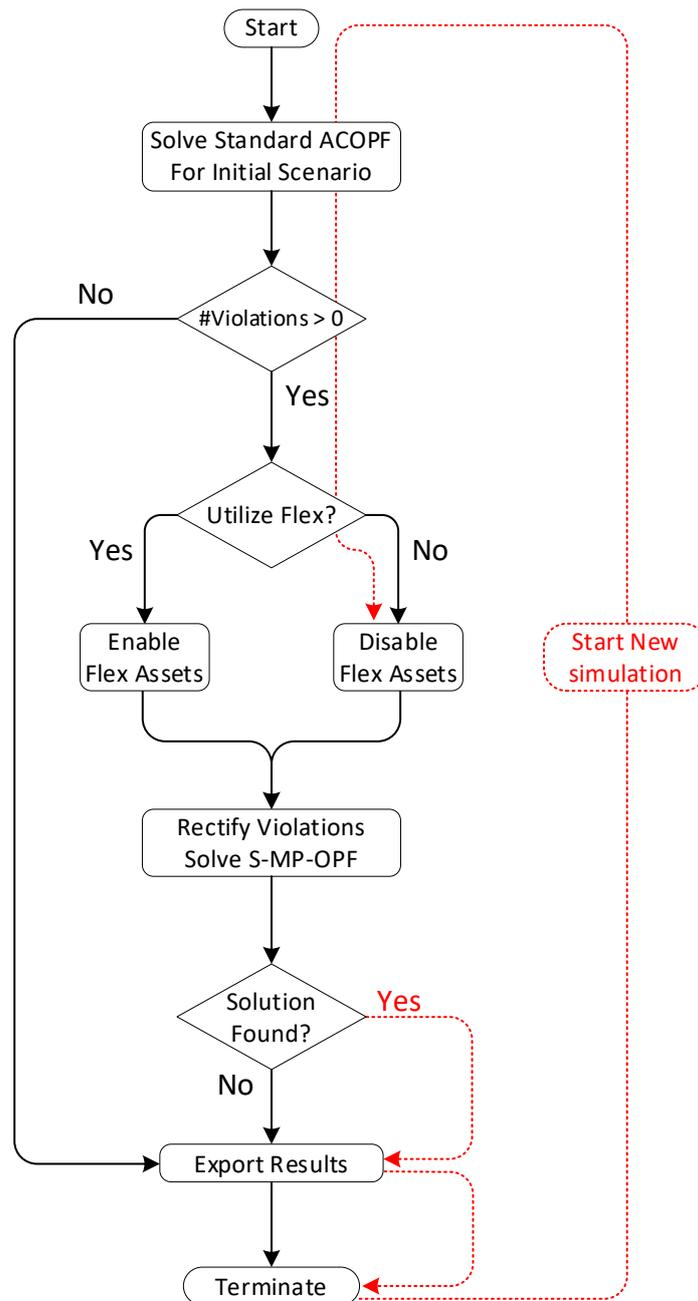
Figure 76 Operation Scenario Handling Approach
