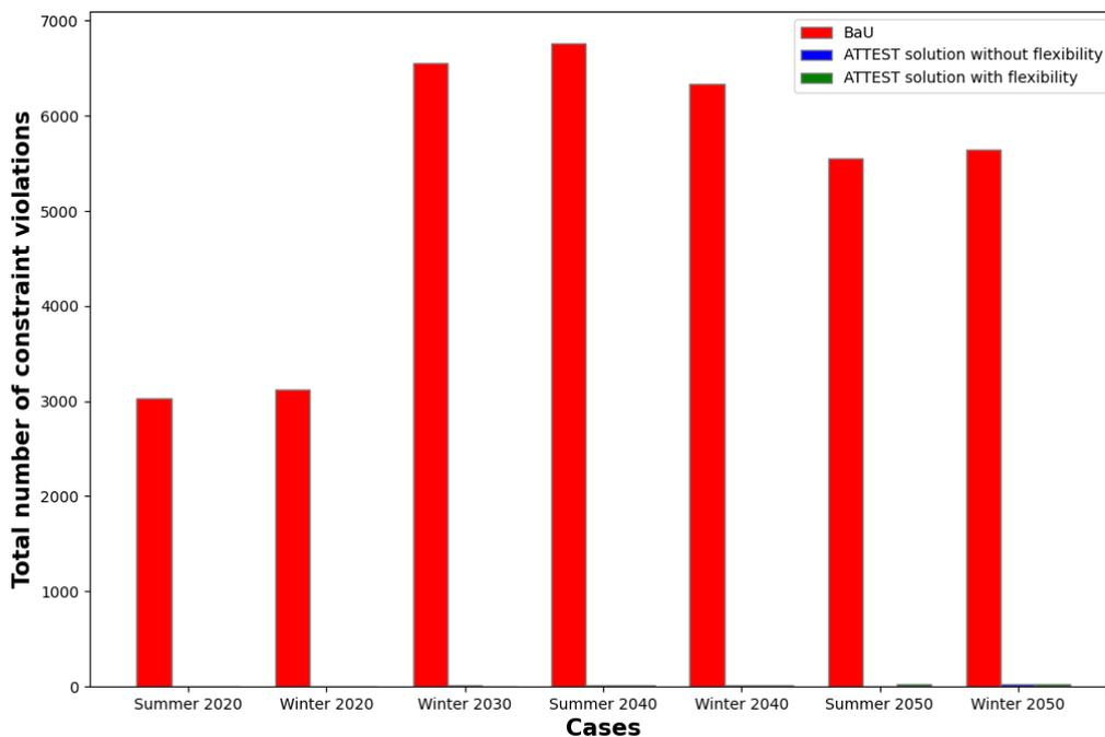
Figure 126 Total constraint violations for representative simulations of the UK network.
