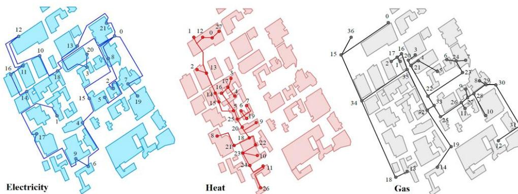
Figure 3 Electricity, heat and gas networks used in the simulations [1]
