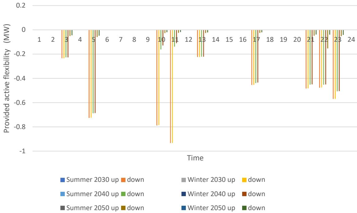
Figure 100 Provided upward and downward active power flexibility from storage units
