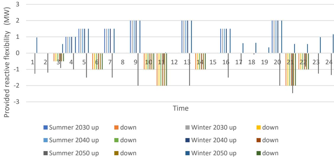
Figure 96 Provided upward and downward reactive power flexibility from storage units
