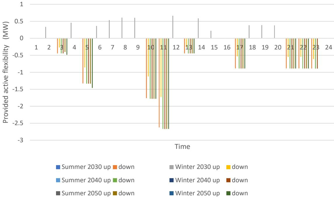
Figure 112 Provided upward and downward active power flexibility from storage units
