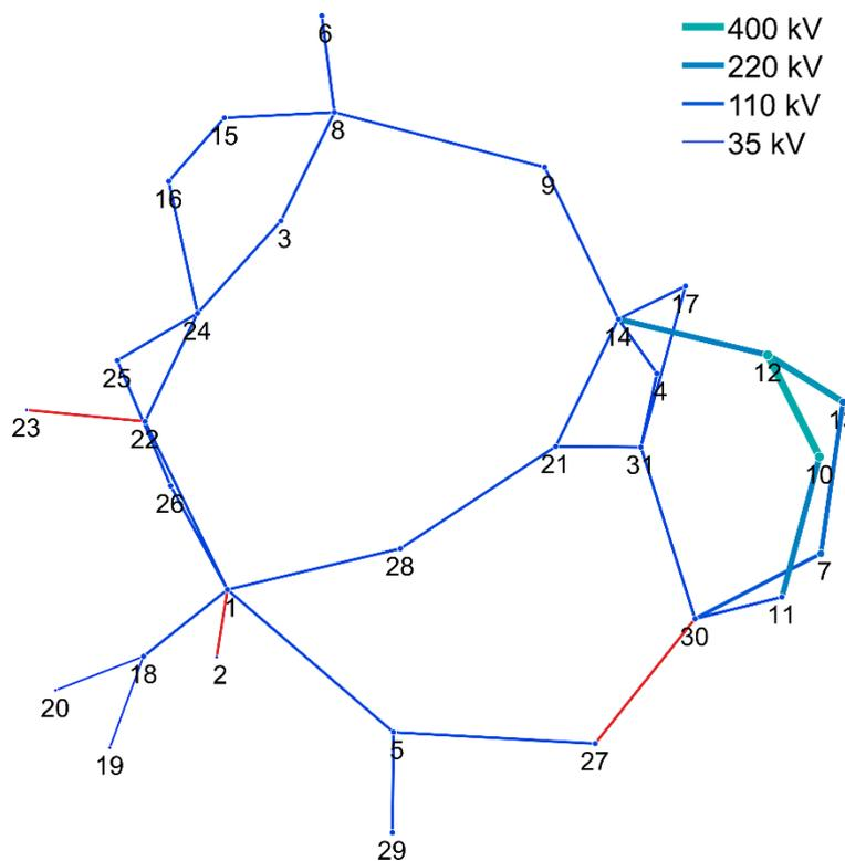
Figure 44 Topology of the Croatian transmission network (HR\_Tx\_01)
