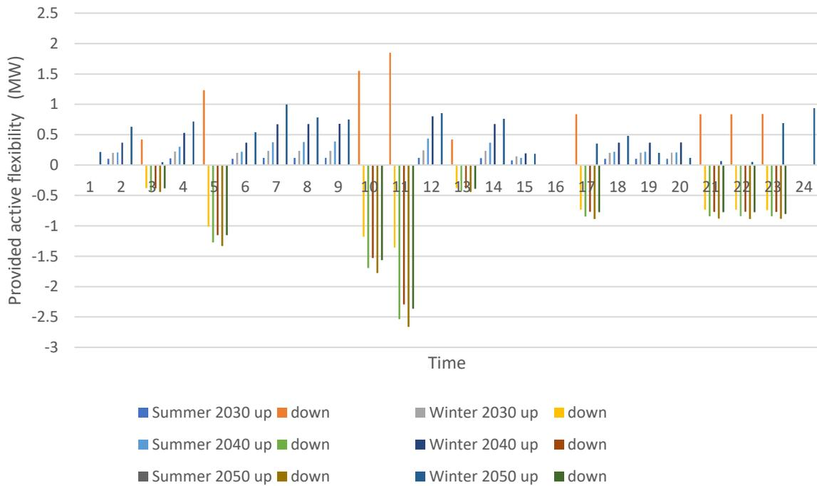
Figure 95 Provided upward and downward active power flexibility from storage units
