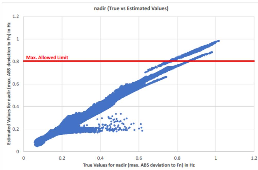
Figure 156 – True vs estimated values for nadir attained after running the tool for all the OPs that composes the TS.
