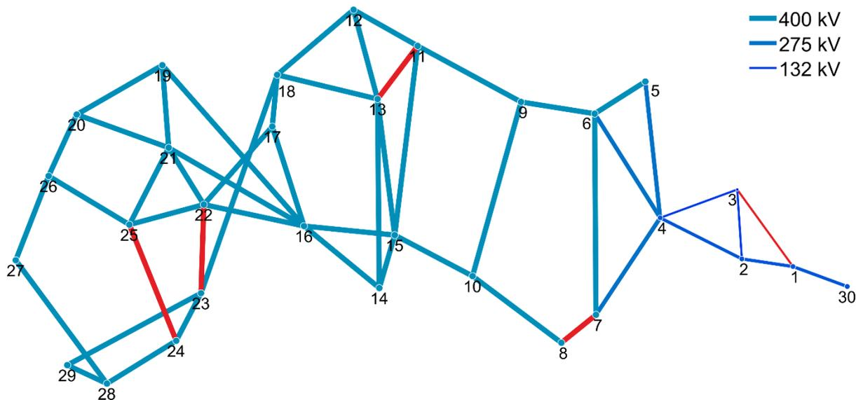
Figure 43 Topology of the UK transmission network (UK\_Tx)
