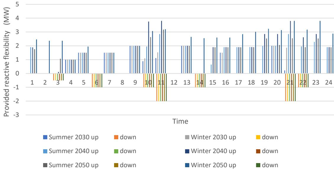
Figure 108 Provided upward and downward reactive power flexibility from storage units
