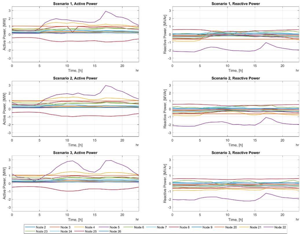
Figure 50 Task 3.3. Case study IEEE. 18-bus DN. Winter consumption profiles, year 2020.
