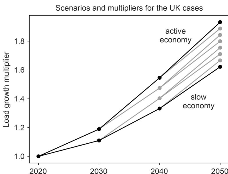
Figure 39 Example of the scenario tree input for the network planning tools: UK load growth scenarios
