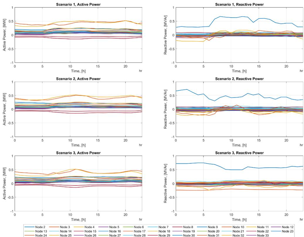
Figure 53 Task 3.3. Case study IEEE. 33-bus DN. Summer consumption profiles, year 2020.
