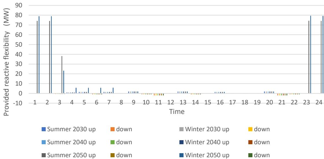
Figure 113 Provided upward and downward reactive power flexibility from storage units
