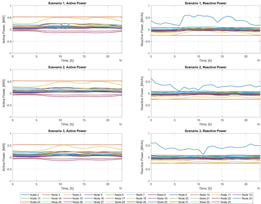
Figure 52 Task 3.3. Case study IEEE. 33-bus DN. Winter consumption profiles, year 2020.
