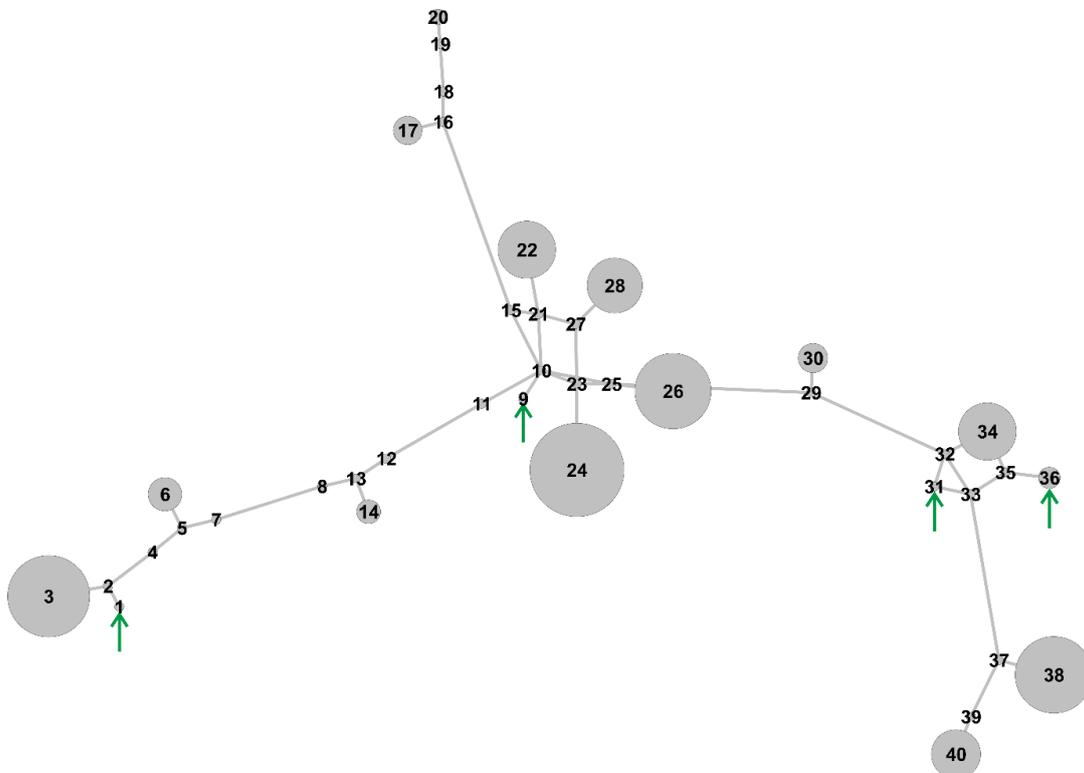
Figure 40 Topology of the Croatian distribution network (HR\_Dx\_01)
