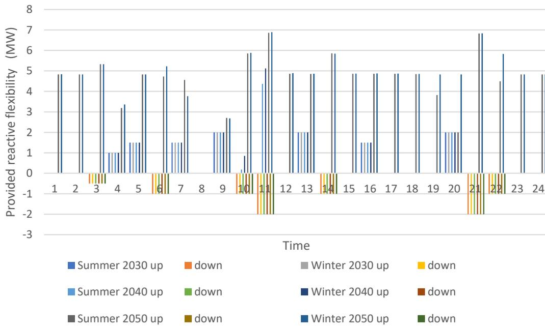
Figure 101 Provided upward and downward reactive power flexibility from storage units
