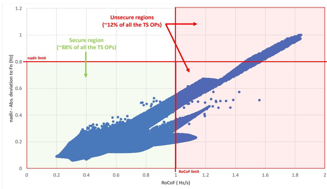
Figure 153 – nadir and RoCoF results (true/real values) attained for all the OPs simulated in the TS and for a three-phase symmetrical short circuit occurred at bus 16 with a clearance time of 250 ms.
