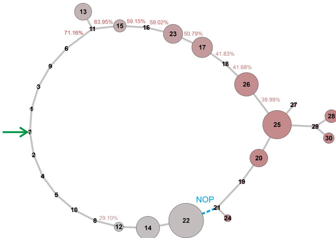
Figure 38 Topology of the UK distribution network (UK\_Dx\_01)
