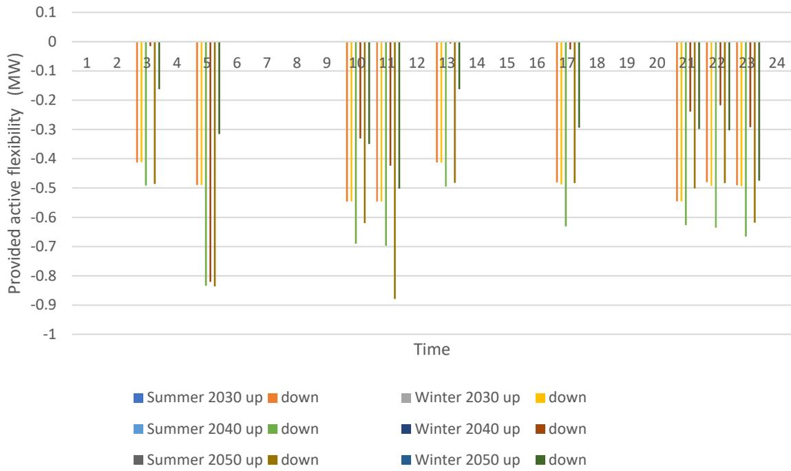
Figure 107 Provided upward and downward active power flexibility from storage units
