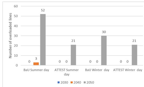
Figure 131 The number of overloaded lines for typical days over the years in Croatia
