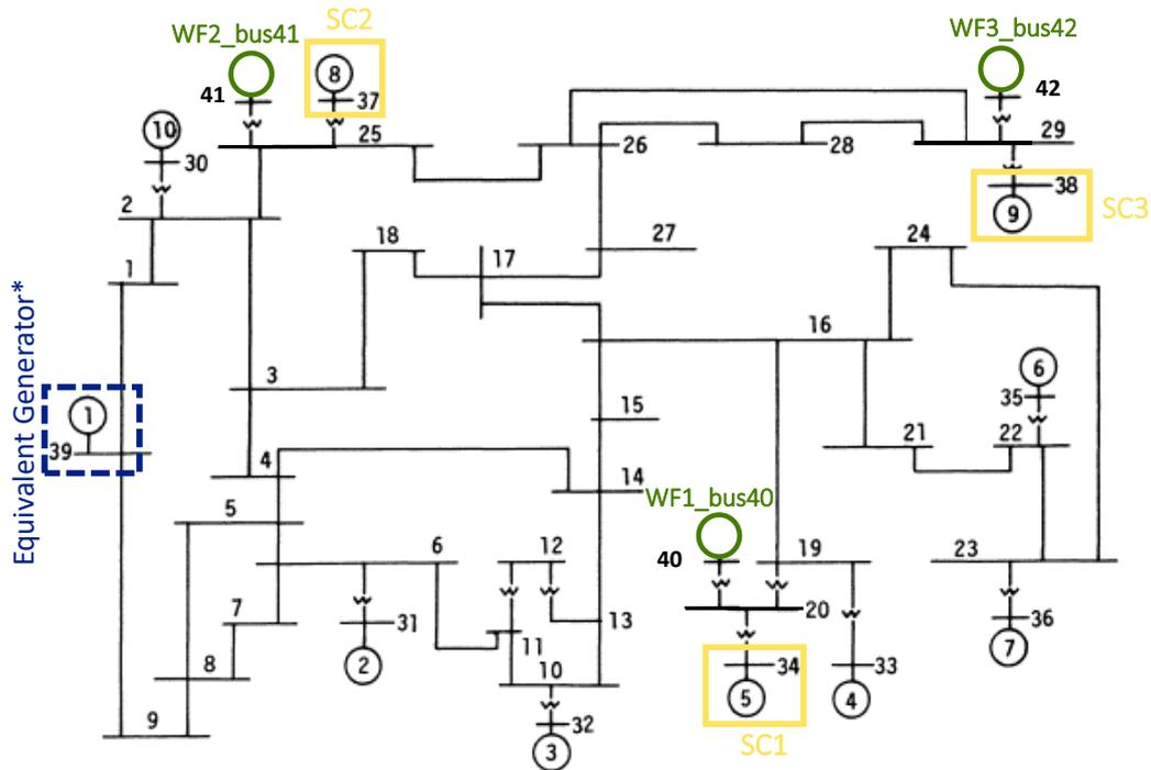
\*Models the remaining interconnected system in terms of all existing synchronous generation units (total inertia) as well as the power flows interchanges with the New England area
