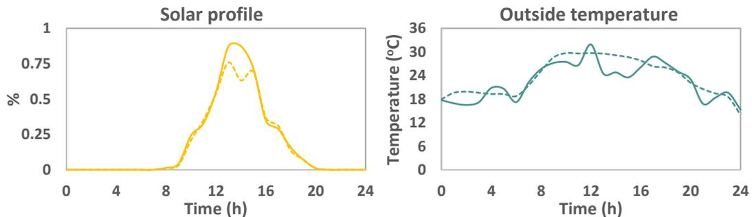
Figure 13 Solar profile and outside temperature forecasts (continuous line) and actual values (dashed lines) during Summer
