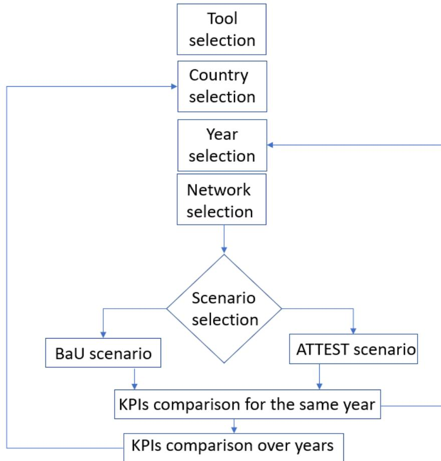
Figure 2 Algorithm for KPIs calculation
