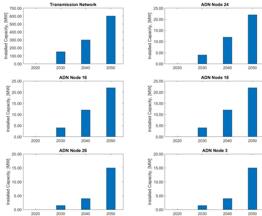
Figure 55 – Task 3.3. Case study IEEE. Total PV installed capacity per network and year.
