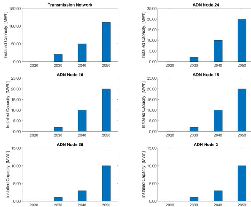
Figure 56 Task 3.3. Total ESS installed capacity per network and year.
