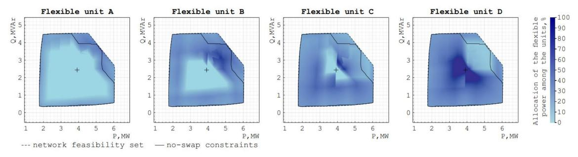
**Note:** The cheapest units get activated more often and are allocated more power and payments **Note:** The power-swap phenomenon happens when multiple units provide flexible power under network constraints
