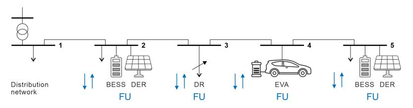
Flexible units – have the technical ability to regulate their power exchange with the grid
